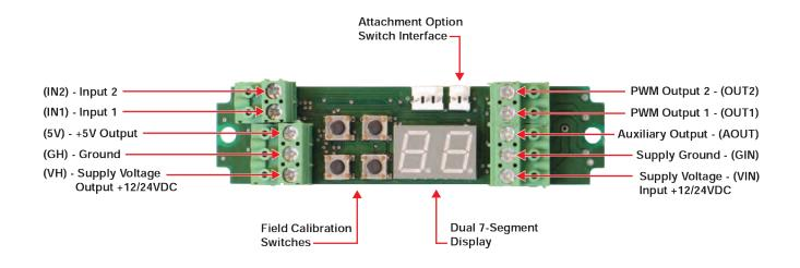
Figure 1: Board Layout and Wiring Connections
