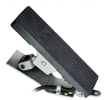
All electronic throttles incorporate our Hall effect sensing or resistive element technology to provide a reliable and durable drive-by-wire signal. Sensors are compatible with all major engine manufacturers and provide a combination of APS and IVS signals which can be factory configured to suit your exact applications.
